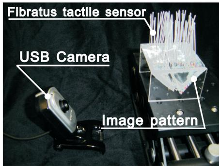
**Figure 8:** Overview of the sensor: The optic axis of the camera is located perpendicular to the captured surface
