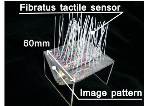
**Figure 7:** Silicone rubber with a lattice pattern: the rubber is transparent and the pattern can be seen. The sensor is almost cube shaped with a side length of 60 [mm]
