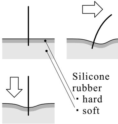
**Figure 3:** Reaction of a fiber: Pressing the fiber along the vertical direction causes a symmetric shift of the silicone rubber. Pressing the fiber along the horizontal direction cause an asymmetric shift of the silicone rubber
