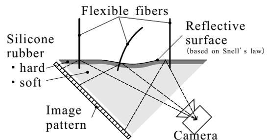
**Figure 2:** *Section of a sensor: Cross-section of the sensor. The surface of the sensor contains some fibers*
