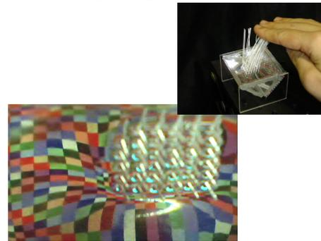
**Figure 10:** After deformation: Acquired image is deformed by the touch toward the fibers
