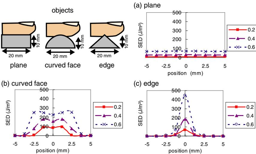
**Fig. 3.** Simulation results. The SED is calculated from  $-5.0 \text{ mm}$  to  $5.0 \text{ mm}$  at  $1.25 \text{ mm}$  intervals. (a), (b), and (c) represent the SED when the fingertip touches the plane, curved face, and edge objects, respectively. The solid, broken, and dotted lines represent SED pushing distances of 0.2 mm, 0.4 mm, and 0.6 mm, respectively.
