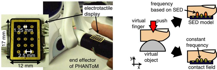
**Fig. 4.** Experimental setup. The left-hand side shows the electrotactile display on the PHANToM. The right-hand side shows the virtual world and the electrotactile stimulus corresponding to the touching condition.
