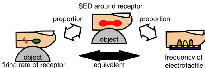
**Fig. 1.** Diagram of the proposed SED model that reproduces the fingertip deformation using an electrotactile stimulus
