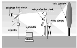
Fig. 15 A schematic diagram of the RPT system used for the optical camouflage in Fig.14.
