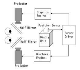
Fig.11 Principle of stereo display using RPT.
