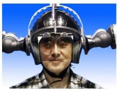
Fig. 12 General view of a Head Mounted Projector (HMP).
