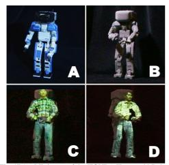
Fig. 17 (A) Miniature of the HONDA Humanoid Robot, (B) Painted with Retro-reflective Material, (C) Example of Projecting a Human onto it, (D) Another Example (adopted from [25]).
