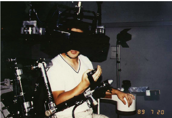
Figure 7: Telexistence Master Manipulation System.
