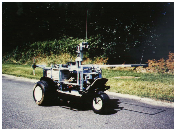
Figure 4: Prototype Mobile Teleexistence Vehicle (Televehicle).
