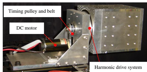
**Figure 2** Experimental joint with harmonic drive system and DC motor
