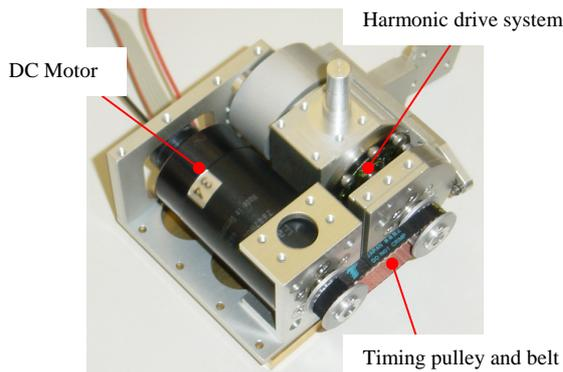
**Figure 3** Drive mechanism used for pitch axis of the wrist
