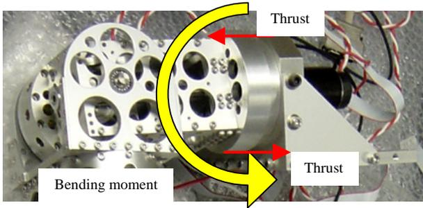
**Figure 6** Forces on the Pitch axis of the shoulder
