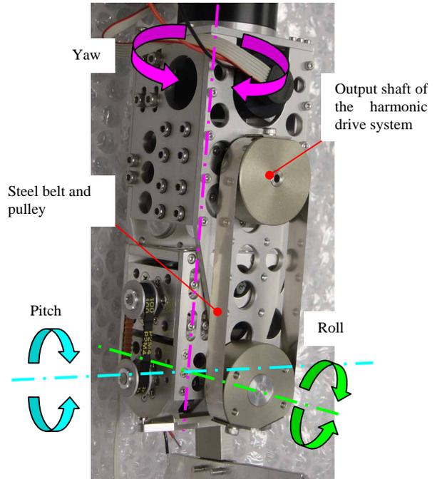
**Figure 4** Mechanism of the wrist joints
