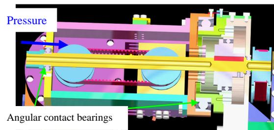
**Figure 5** Position of angular contact bearings
