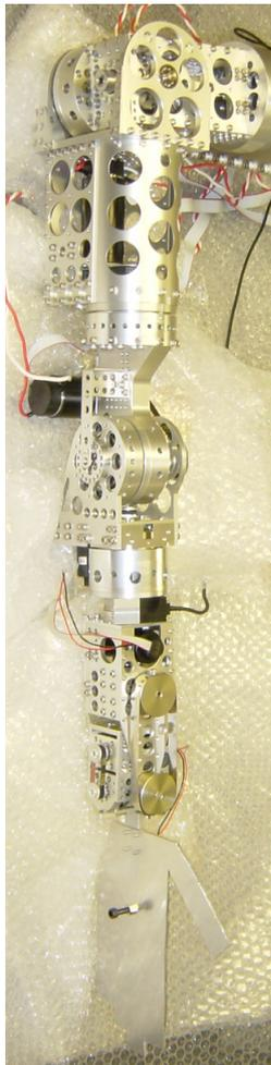
**Figure 1** Complete view of the 7-DOF arm
