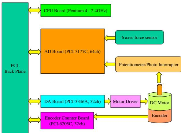
**Figure 7** Control system for the arm
