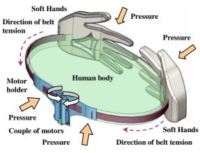
Fig. 2. Structure of wearable HaptiHug device
