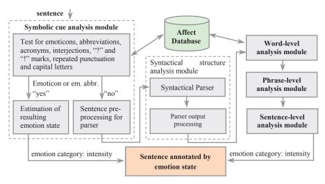
Fig. 2 Working flow of the Affect Analysis Model.
