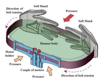
Fig. 6 Structure of wearable HaptiHug device.
