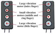
Fig. 10 HaptiTickler device.
