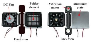
Fig. 9 Structure of HaptiShiver/HaptiTemper.
