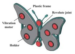
Fig. 8 Structure of HaptiButterfly.
