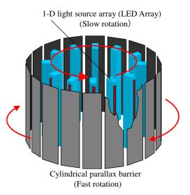
Figure 1: Schematic diagram of basic structure
