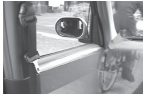
Figure 2: Implementation on a car:the door seems transparent.
