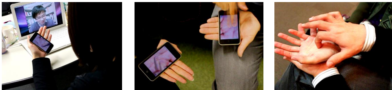
Figure 1 Remote tickling with video chat (left). Users can observe a moving fingertip, which looks like someone is actually tickling the palm with his/her fingertip (center). Tickling as a physical contact (right).
