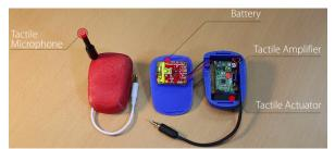
Figure 3: Attachment overview: microphone includes an embodied probe; captured signals convey audio through a jack attached to the smartphone; the vibro-tactile wave is displayed using a tactile actuator though a tactile amplifier from the smartphone.
