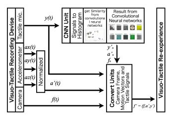
**Figure 6**: Proposed architecture for displaying recorded data and recognizing vibro-tactile waves. In this case, we used a convolutional neural network.
