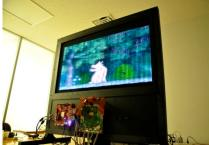
Figure 1. The 38-inch adaptive parallax autostereoscopic LED display
