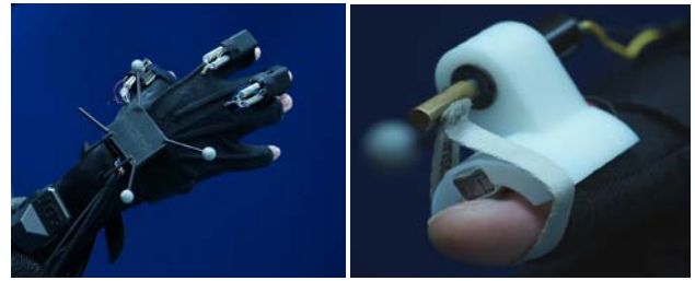
Figure 5. The haptic glove (Left) and display mechanism to reproduce pressure and vibrotactile sensation (Right)
