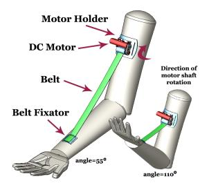
Figure 2. FlexTorque on the human's arm surface.
