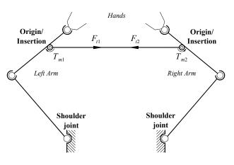
Figure 12. Kinematic diagram of FlexTensor and human arm.
