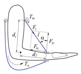
Figure 4. Diagram of applied forces and torques.
