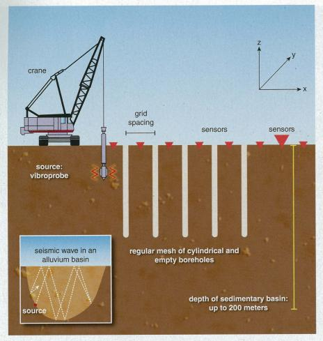
The basic idea behind seismic cloaking is to alter the density of the medium, causing the waves to change speed and, by extension, direction, so they go around a target. A recent experiment demonstrated that a series of precisely spaced bore holes could effectively change the direction through the ground of vibrational waves produced by an artificial source. (Adapted from Brûlé et al., 2014.)
