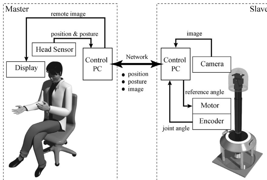
Figure 2. TORSO system diagram.
