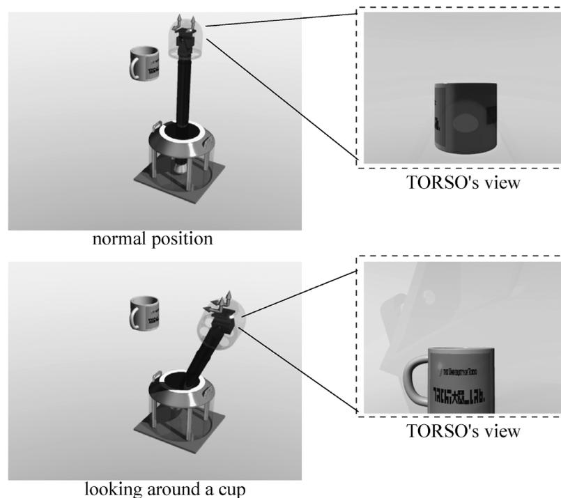
**Figure 1.** Motion involving looking around an object.
