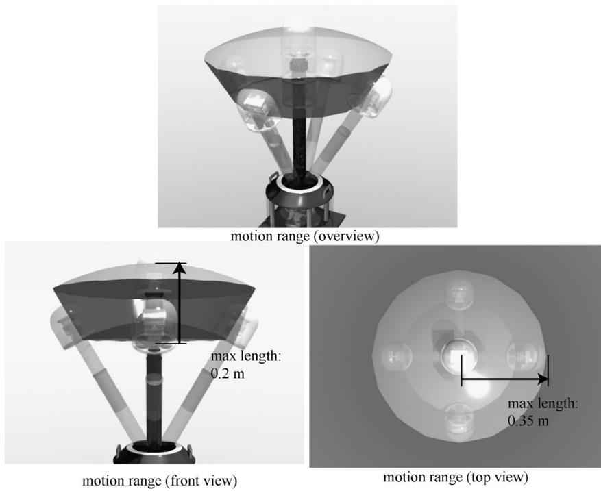
**Figure 7.** Extension of the field of view.
