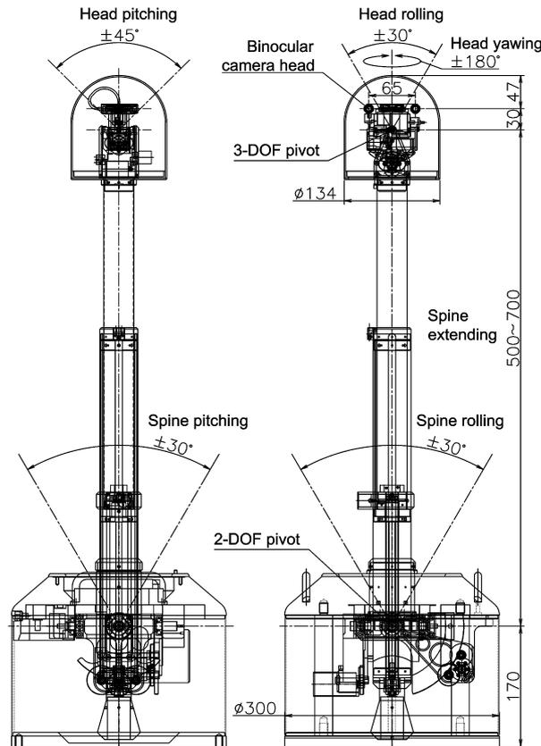
**Figure 4.** Schematic of TORSO.
