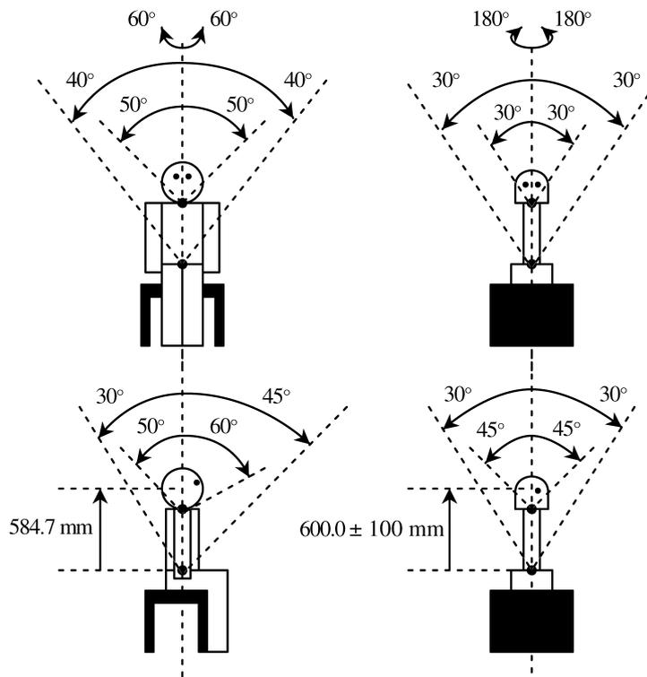
**Figure 6.** Motion ranges of the upper body of humans and TORSO.
