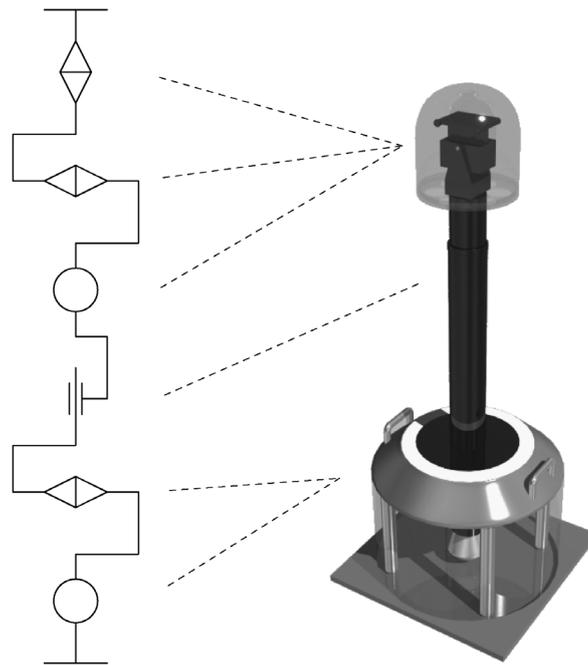
**Figure 5.** The d.o.f. arrangement of TORSO.
