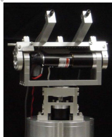
Fig. 2 TELESAR II slave head
