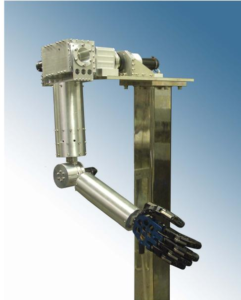
Fig. 1. Developed whole-sensitive robot arm.
