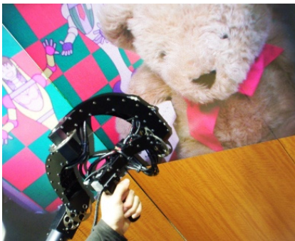
Fig.15: View from operator's eye using HMP without a retro-reflective cover on master arm
