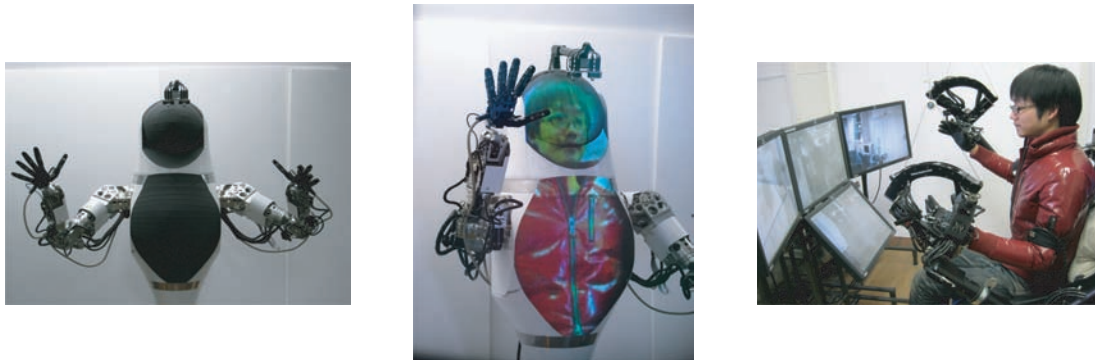
Fig. 12 Example of RPT view (left: TELESAR II without projection; center: with projection of an operator; right: operator at the control).
