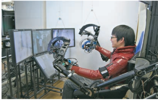
Fig. 7 Acceleration sensor attached to operator's upper arm along swivel axis.
