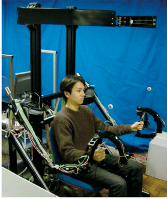
Fig. 5. The master arm of TELESAR II.
